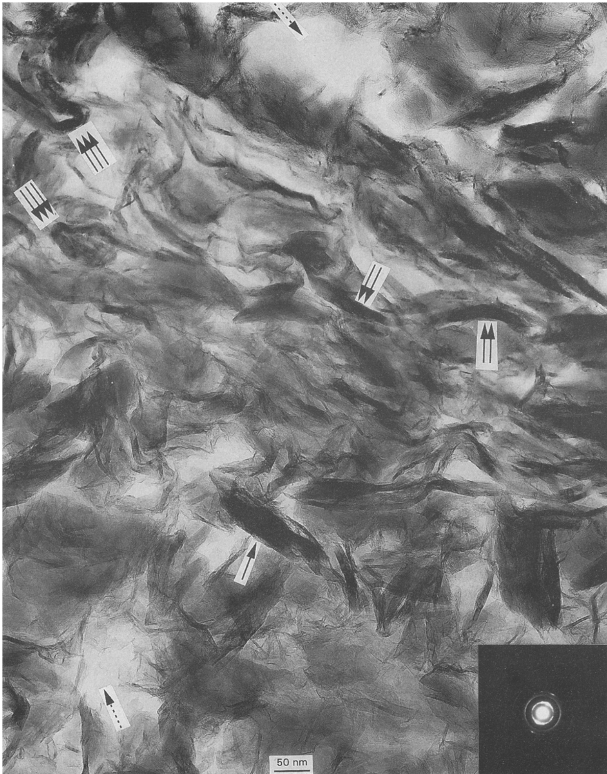
Figure 10 High-magnification TEM bright-field image of the transverse section in the graphitized fibre spun at 295 °C.
