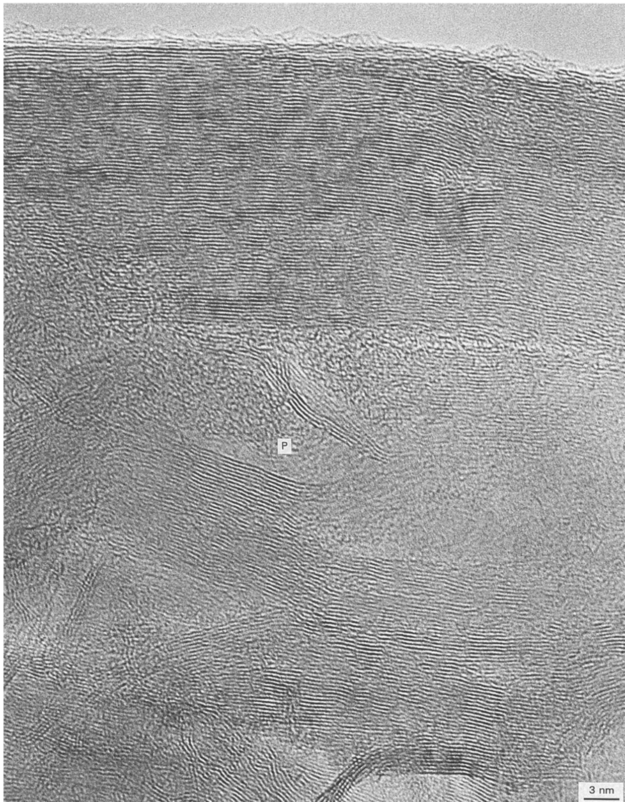
Figure 14 TEM lattice fringe image of the longitudinal section in the graphitized fibre spun at 295 °C.
