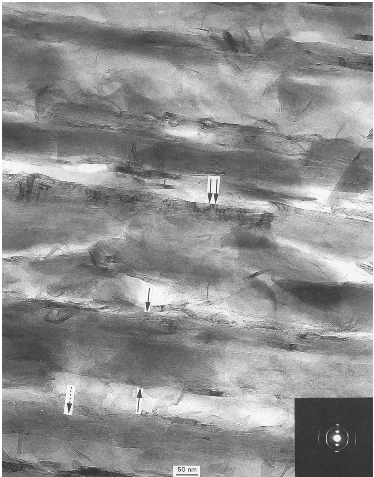
Figure 12 High-magnification TEM bright-field image of the longitudinal section in the graphitized fibre spun at 295 °C.
