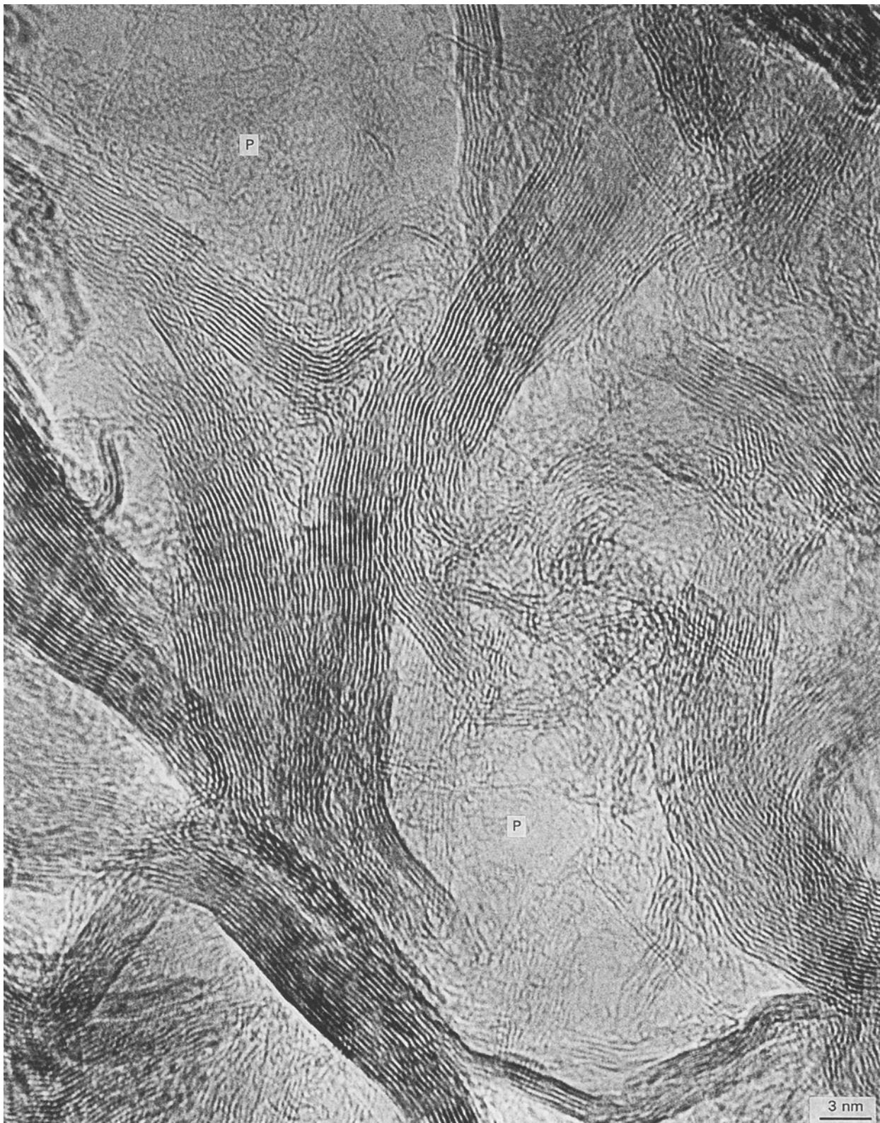
Figure 11 TEM lattice fringe image of the transverse section of the graphitized fibre spun at 295 °C.
